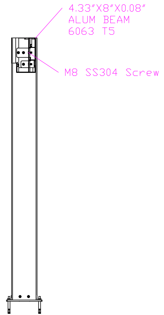
SECTION A-A LOUVER BEAM REINF. DETAIL
